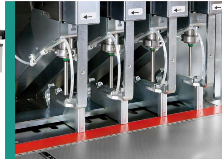
Professional drill bit lubrication with cooling system
